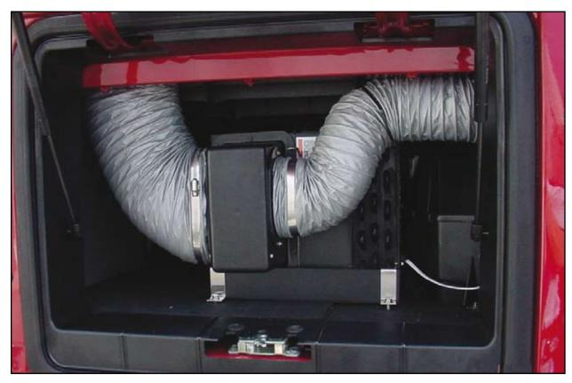
Figure 15. View of supply ducting connected.
